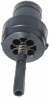
FIST Gel Sealing Kit for round splice closure port, sealing 4 cables with diameter between 4 and 7 mm
