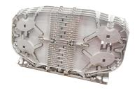
FIST<sup>TM</sup> Splice Sub-assembly kit for GCO2-FC/FD flat closures with 4 slim High Density (HD) element trays, each for holding up to 24 primary coated fibers, with Heat Shrink type splice holder
