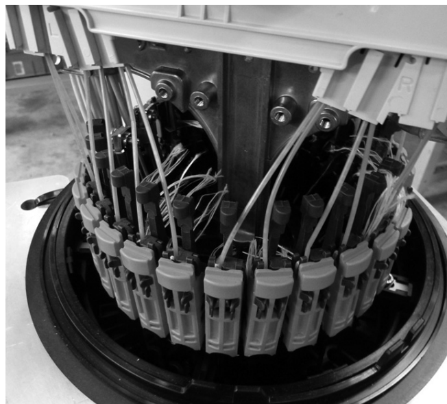
4.3.22 Routing of the cables towards tube holder.
