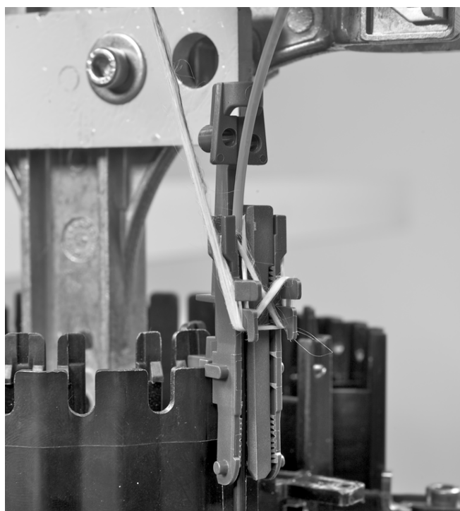
4.3.18 Wrap the aramid strength member as shown.
