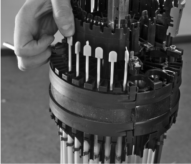
6.1 In case of unused ports apply the yellow plugs to seal the ports. Note: The blind plugs need to be inserted from inside.
