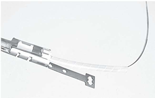
4.2.35 Insert the spiral tube over the fibers into the breakout till the tube stop. Open the round port and place the heatshrink as discribed in loose tube preparation.
