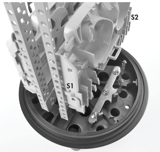
**16 PORT BASE:** Ports (1+3+5+11+13), (2+4+6+12+14) for cables to (S2). Ports (5+7+9+15+17), (6+8+10+16+18) for cables to (S1). Verify the position of two cables if they are placed on the same side (next to each other) because the total amount of loose tubes in ports going to one tubeholder can never be more than mentioned in the capacity of the tubeholder.
