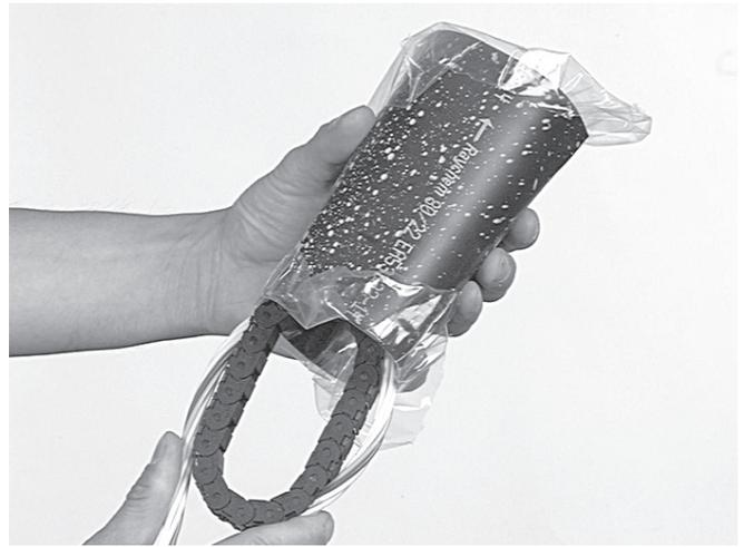
4.1.10 Take the oval sleeve and place the packing bag that has been opened on both sides in the oval sleeve to protect the hotmelt inside the sleeve against dirt and grease. Take the LCIT and bend the loose tubes gently over it. Push the loose tubes in the sleeve. The non-coated edge of the sleeve (arrow) should be pointed to the base of the closure.
