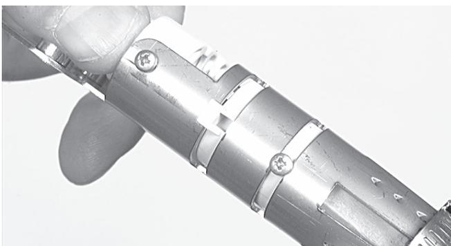
4.2.25 Slide the loop breakout device in the loopbracket and secure the two screws. Open the oval port as described in loose tube preparation. Take the oval sleeve and place the packing bag that has been opened on both sides in the oval sleeve to protect the hotmelt inside the sleeve against dirt and grease. as described in loose tube preparation.
