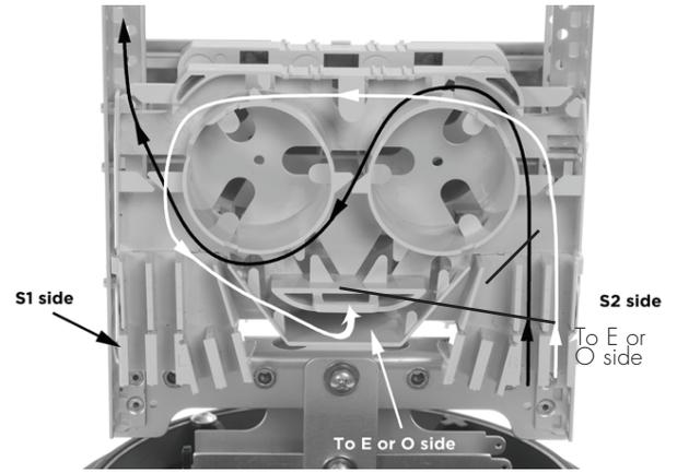
Fibers can be routed between OS1, OS2, ES1 and ES2. In case that fibers have to be routed from SIDE-O (Odd portnumbers) to SIDE-E (Even portnumbers), use the window (see picture). Select the cable termination as such, that a minimum of fibers will cross and have to be routed through the window. Therefore the selection of the ports according to the cable lay-out is important.
