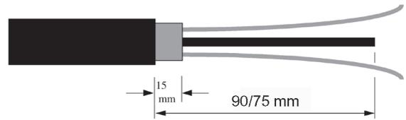
4.1.22 Remove the strength member leaving 90 mm from the cable jacket, if shield present leave 15 mm of the shield.
