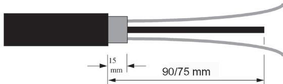
4.1.27 If big ports 3-4-5-6-7-8-9-10 are used, cut strength member at 90 mm length. If small ports 11-12-13-14-15-16-17 and 18 are used, cut strength member at 75 mm length.
