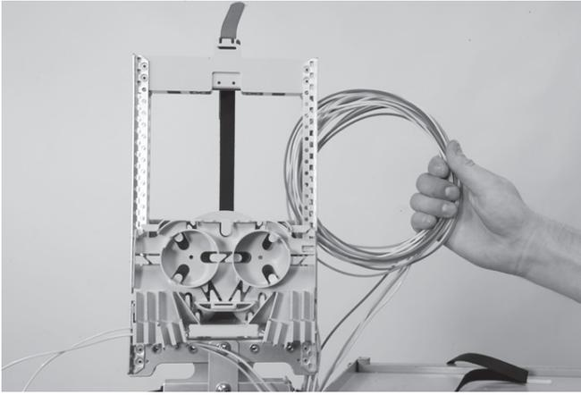
4.1.14 Make some loops with the uncut loose tubes, and put these in the plastic bag (Be careful not to damage the loose tubes!). Two sizes of bags are available. Use the correct size according to the volume of the loose tubes.
