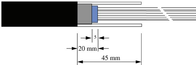
4.2.29 Remove the jacket for **45 mm** leaving the strength members. Be cautious not to damage the strength members. In case of metal shield, remove 5 mm from the end.
