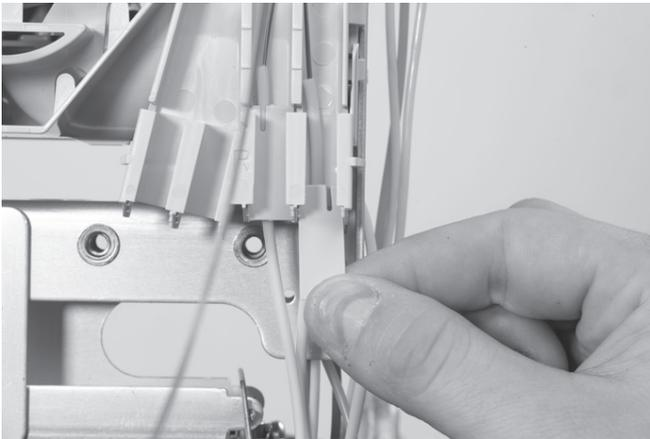
4.1.18 In case of **Reversed oscillating cable** Identify exchange and customer-side using some PTFE tape around the fibers. One can also use the FIST-split-collets-rings markers to identify the loose tubes.
