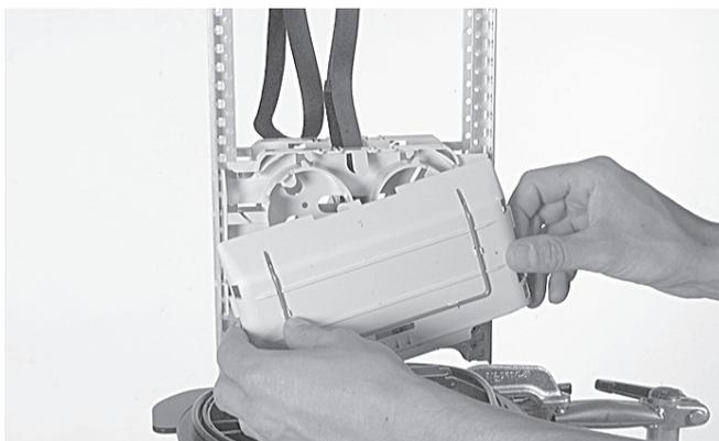
6.1 Remove the hook and loop fastener and routing block cap. To remove the routing block cap lift the two snaps at one side of the routing block cap.
