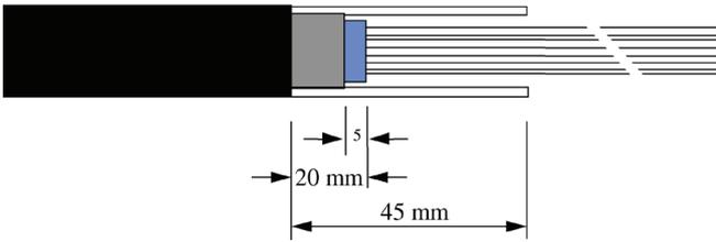
4.2.3 Remove the jacket for 45 mm leaving the strength members. Be careful not to damage the strength members.
