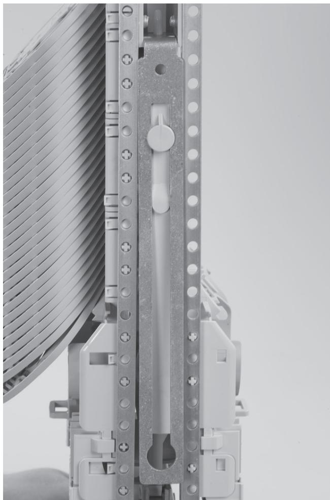
4.2.23 Secure the basket by mounting the metal profile on basket and closure bracket.
