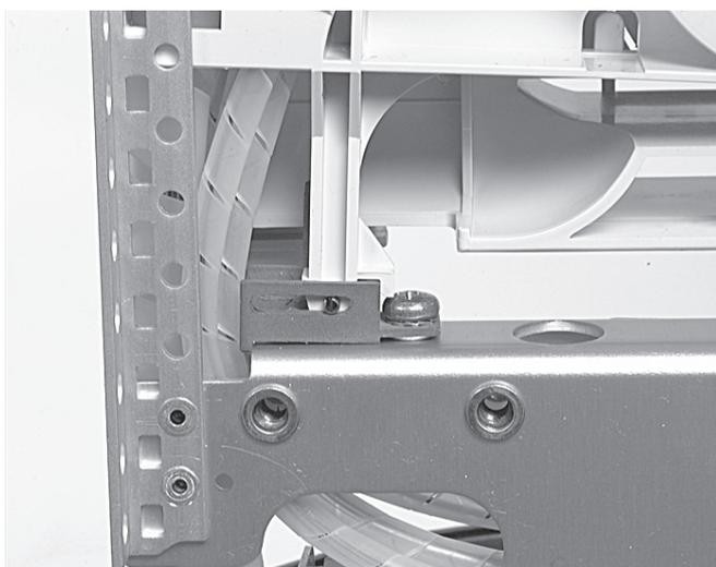
4.2.22 Place cover back in place, Make sure the cover is under the lip of the bottom island. Hinge the basket inbetween the UMS profiles and make sure the hinge is in the correct position.
