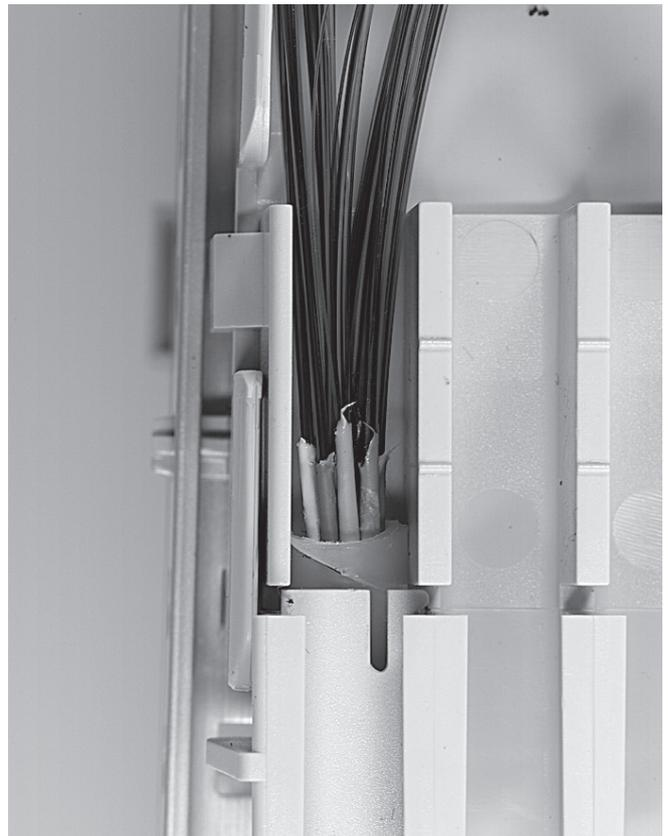
4.2.27 Match the spiral tube on the tubeholder, mark and cut the spiral tube from this mark. Remove element per element the ID cords or compact cable sheet (Microgain™, Compacttube™, ...) till about 10 mm after the spiral tubes; use PTFE tape to bundle the fibers and the ID cord. Position the small spiral tubes in the respective tubeholders. Bottom picture shows compact cable sheet.
