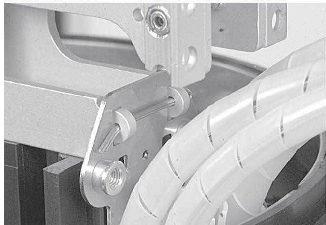
4.2.9 Position the loopbracket in the bottom bracket and lock with the split pin.
