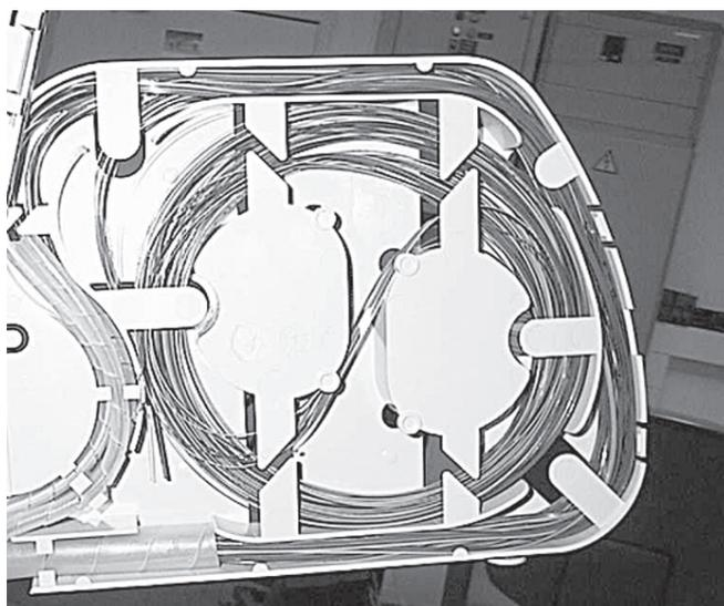
4.2.16 **All** fibers are placed in the “fiber twist storage duct” as shown on the figure above. **One has to place the fibers as far as possible at the outside of the path** because when closing the basket some overlength will be pulled out of the basket (risk of loading fibers when basket is hinged).
