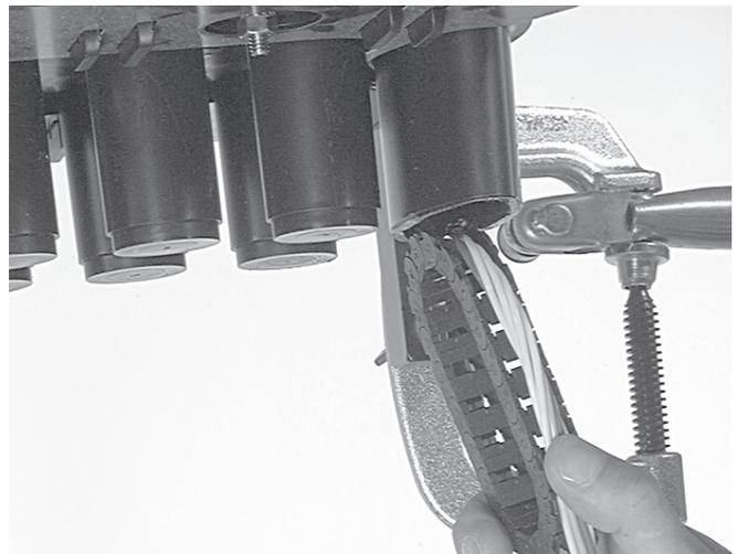
4.1.11 Push the loose tubes (looped around the LCIT) through the oval port. Remove the LCIT and pull the cable gently in the closure.
