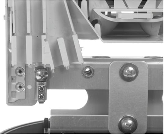
4.1.23 Secure the strength member connector in the closure (on the bottom bracket )
