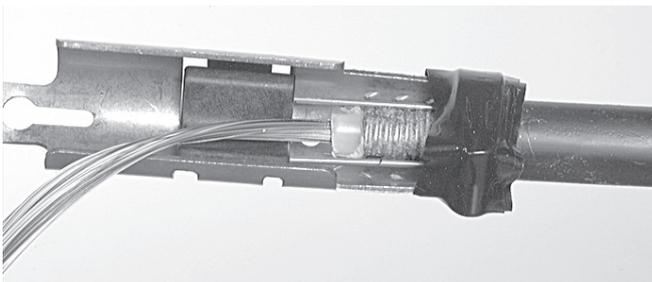
4.2.33 Insert the strength members from the cable into the strength member stop. Secure the cable with the hose clamp in case cable diameter is more than 8 mm. onto the bracket. Secure the cable with tie wrap in case cable diameter is less than 8 mm. onto the bracket. Secure the screw of the strength member stop on the bracket. Wind a few layers of tape around the hose clamp.
