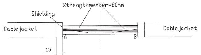
4.1.4 Remove the strength member leaving 80 mm from the cable jacket, if shield present leave 15mm of the shield
