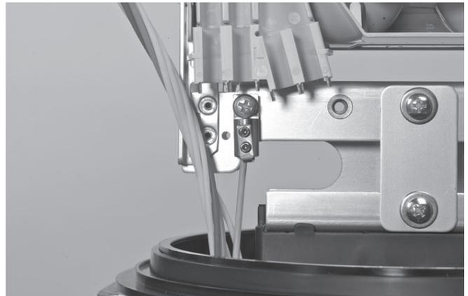
4.1.25 Push the loose tubes in the port and secure the strength member in the strength member connector. Be sure that all loose tubes are routed without crossing around the strength member.
