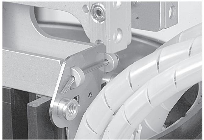
4.2.26 Push the fibers in the oval port and position the loopbracket in the bottom bracket and lock with the split pin.
