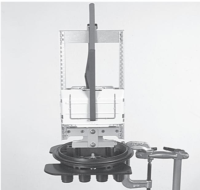
3.1.1 The FIST-GCO2 will be mounted temporary on the work-stand. The work-stand is wrap-around, so that the FIST-GCO2 installed with cables can be taken away from it. Secure the FIST-GCO2 base onto the workstand with the four split-pen.
