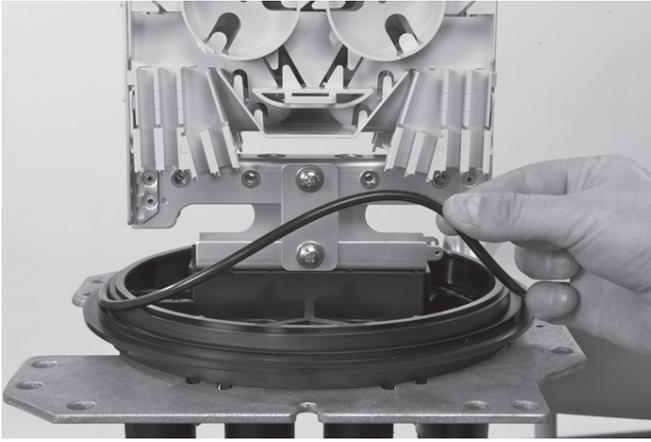
3.2.1 Open and remove the clamp. Remove the dome and the O-ring
