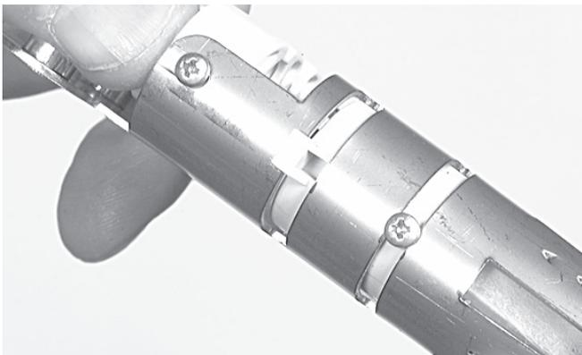
4.2.6 Slightly loosen the screws of the two strength member stops on the loopbracket such that one can position the strength member stops according to the position of the strength members.
