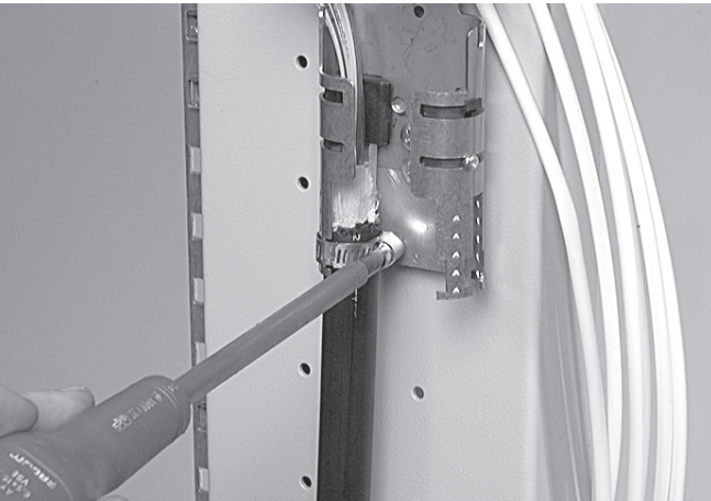
4.1.14 Secure with the cable clamp. Don't squeeze the cable.
