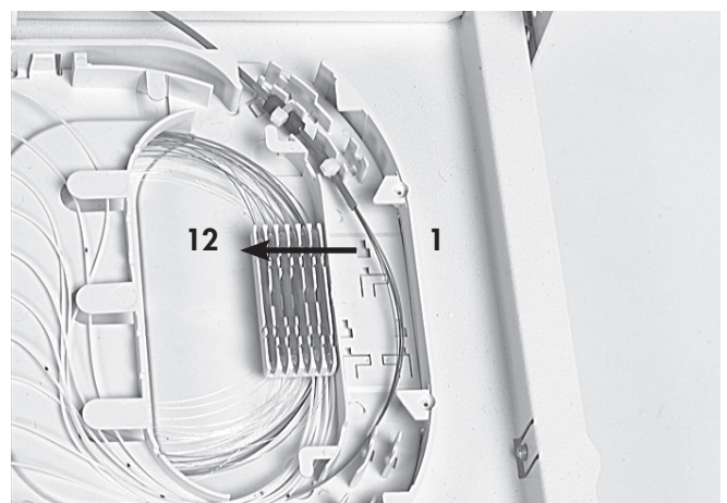
5.1.10 Place the splice protector in the holder, start at outside of the tray, (hold the splice holder with finger to prevent bending) and coil the fibers in the tray.
