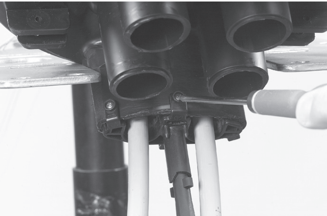
3.2.7 Tighten the 4 screws, make sure they grip in the port.
