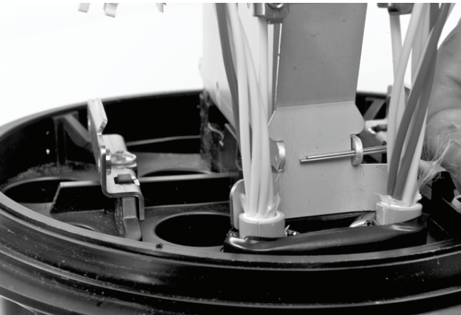
3.4.6 Install the metal bracket to the frame and secure with split pin. Secure the strength members. Install the spiral tube over the loose tubes.
