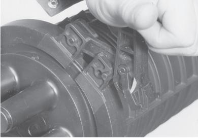
**9.4** Place the dome carefully over the trays onto the base. Put the clamp around the base/dome interface. Close the clamp.
