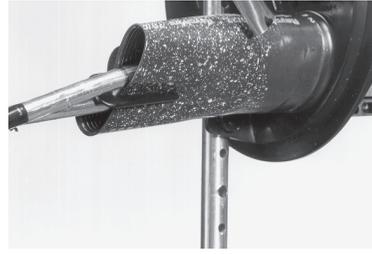
**6.6** Shrink the oval cable seal on the FOSC-base side with the recommended hot air gun device with reflector. Shrink sleeve until the green thermo-indicating paint is converted to black. (Make sure the hot-air temperature is at least 350°C). (If a FACC-HEAT-GUN-220V is used, set position on scale 10).
