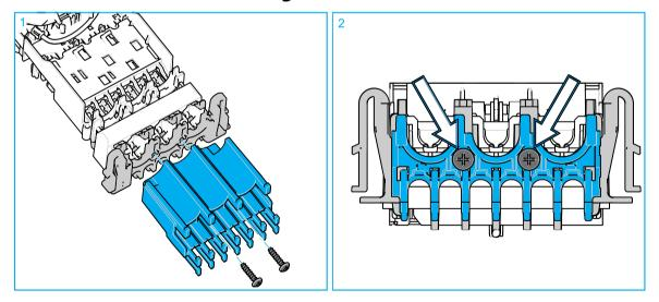
1 Secure the external cable guidance bracket onto the organizer of the CC 100/40 with the two screws.
