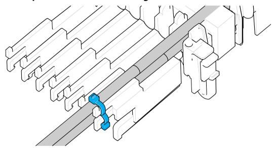
Secure the drop cables to the external cable guidance bracket using cable ties.
