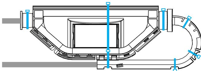
2 Secure the fiber cable with the cable ties.
