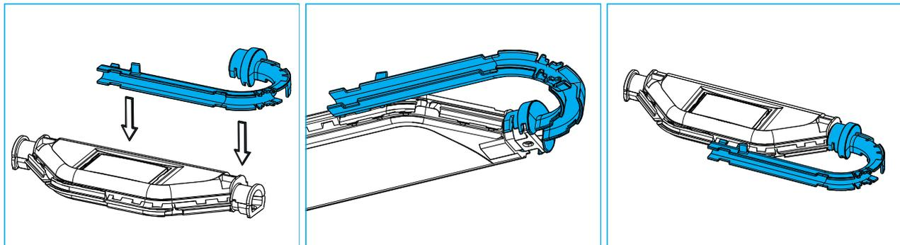
1 Install the fiber cable guide as shown in the pictures above until it snaps onto the SRC10.
