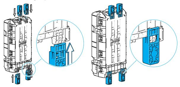
Mount the clips on the base on the 4 positions as shown.
