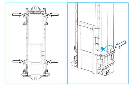
1 There are 4 locations to secure the closure with a securuty wire. Push the wire through the holes on the top and bottom cover and seal the wire per local practice.
