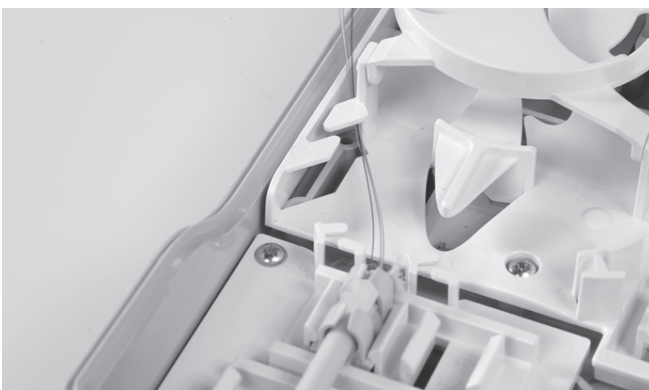
2.3.1 Route the fibers to the storage area. All fibers should enter through this port.
