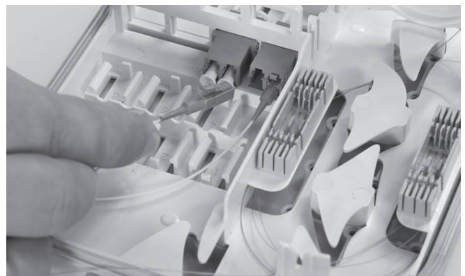
2.3.3 Connect the pigtails into the designated adaptors.
